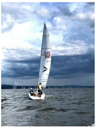
Some design specifications: 18 ft. length overall, 14.2 ft. length at the waterline, 1240 lbs. displacement, 700 lb lead keel. The keel makes it a stable boat. The elliptical, narrow keel and rudder give the boat good handling and pointing ability. The boat remains mostly dry even when heeling 20 degrees.
