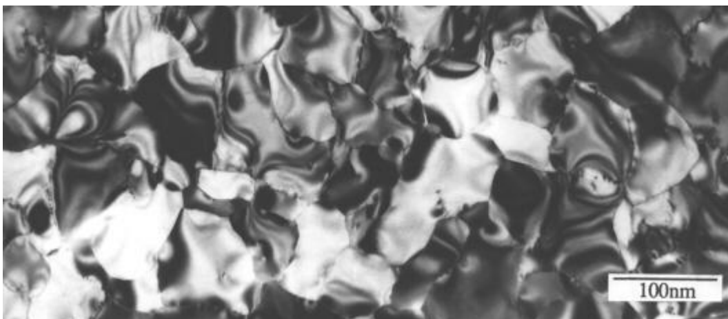
Plan view TEM image confirming the distribution of rotated grains.
