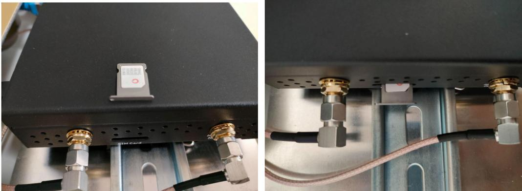
SIM should be **facing upwards** when inserted. Push SIM tray all the way in until flush with the case (not shown)
