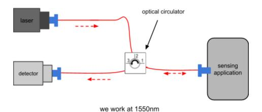
This would work very well with SM-PM fiber. A true optical circulator cannot work with MultiMode fiber or non-PM fiber.
