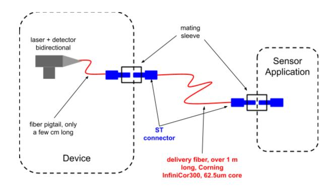
A laser signal is emitted by the laser (see *laser + detector*) and transported to the *Sensor Application*. From the sensor application the laser signal is sent back through on the same path towards the detector (see *laser + detector*). There are some optical connections in between.
