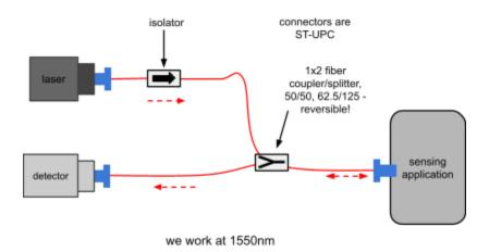
This was built with the Chinese photonics parts. (see <u>specs for LD + Isolator</u>), tested, but doesn't work properly because it gets too much signal back into the LD and makes that LD fluctuate. The MM fiber doesn't preserve polarization.
