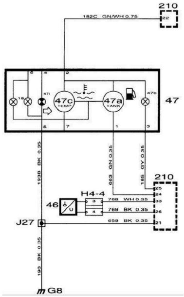
When the ignition switch is in the Drive position, 12 V is supplied to pin 2 of the temperature gauge from pin 22 of EDU 210. Fuel level sensor 46 is connected to the EDU unit which performs a calculation and sends a 1-9 V signal to pin 1 of the tank/temperature unit.
