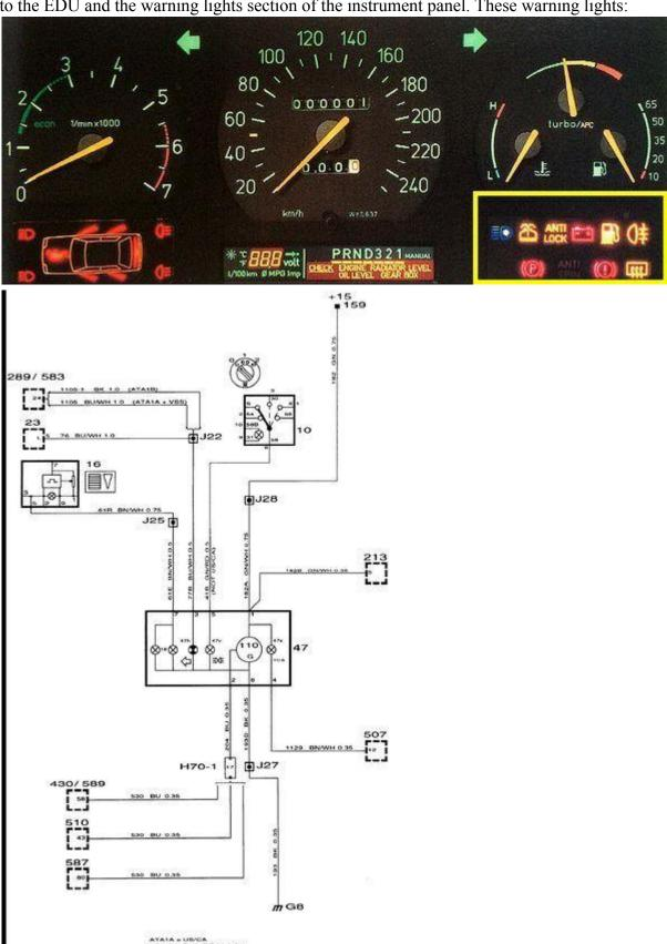
Schematic and brief explanation of the "Combined Instrument" (i.e. the fuel tank & coolant temperature gauges):
