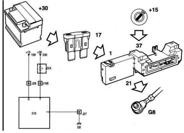
They fail to mention that after the ignition switch, the +15 is fed through fuse #13 - and then to the EDU and the warning lights section of the instrument panel. These warning lights:
