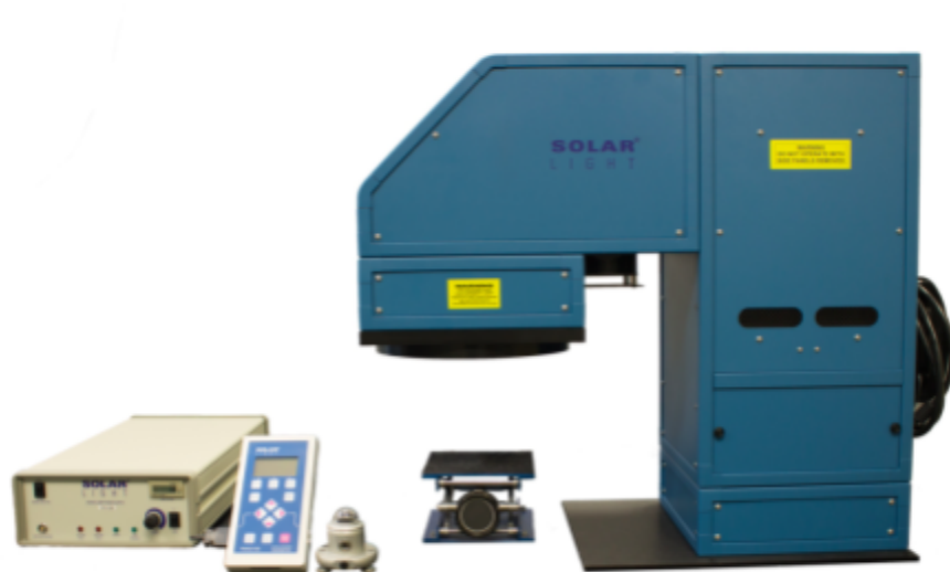
Figure 18. Simulator, Pyranometer, radiometer, power supply set-up [88]
