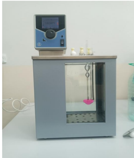
Figure 1. TV12LT Low Temperature viscosity bath (low-temperature thermostat bath)
