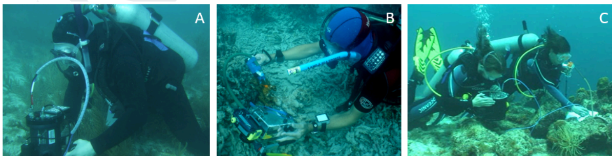
Figure 3.5 Hand-held underwater spectroradiometer systems with fiber optic probes A) once commercially-available Night-sea unit with artificial illumination in a closed path system; Photo credit: H. Dierssen B) single diver unit with artificial illumination and a fibre optic cable; Photo credit: C. Roelfsema. C) two divers operating a handheld system with ambient solar illumination. Photo credit: Jeff Godfrey (UConn).
