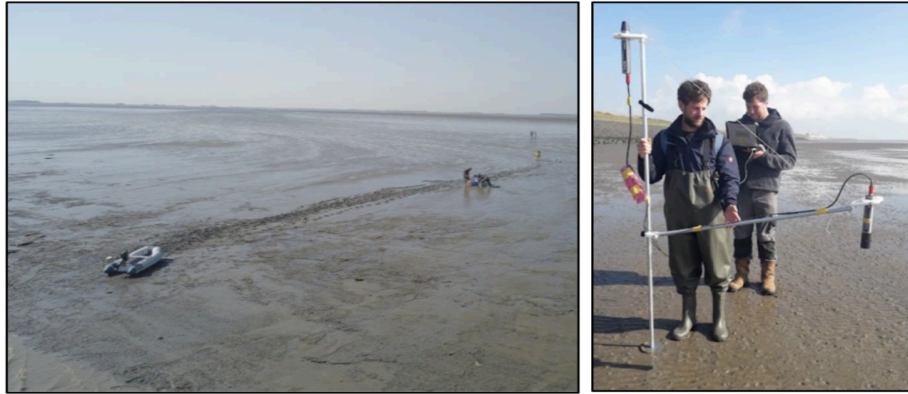
Figure 7.2 A) Drone image of a sampling group at the Heringsplaat, Netherlands. The group arrived on a rubber boat that was stationed on the mud. B) Sampling gear for measuring downwelling irradiance and upwelling radiance over the mud flat. Photo source: J. Pitarch
