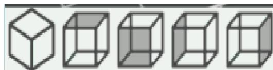
From left to right in order: Isometric view, top view, front view, left view, right view.
