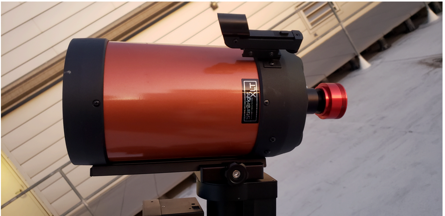
Figure 10: Existing Imaging train on an assembled observing system. Note the simple connection between visual back, nose-piece, and camera. Note that while this is a simple imaging train, other equipment combinations may have more complex considerations. If using an optical reducer or corrector, certain back-focus (distance from camera to corrector) requirements must be met. Additionally the use of any filters or guiding equipment will complicate the imaging train as well.
