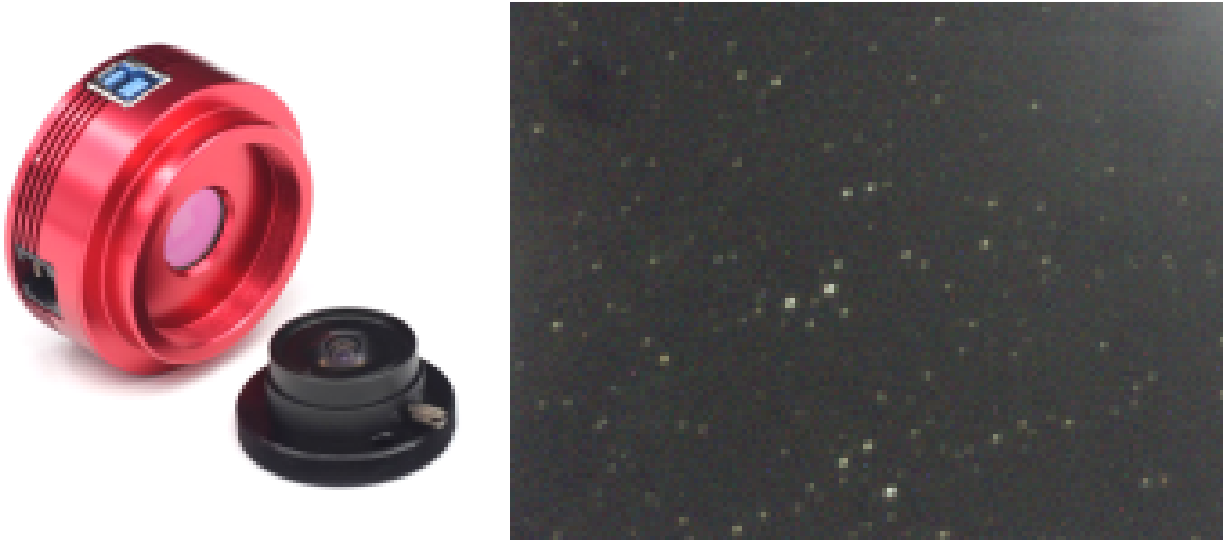
Figure 9: (Left) The ASI224MC "hockey puck" camera. The heart of the camera is the imaging sensor (shown in the center) which is supported by a round housing with a USB3 and ST4 cable port. The front of the camera is threaded to allow us to easily attach it to our imaging train. (Right) An example raw image taken with the ASI224MC. Note that your images will be monochrome before the process of debayering.
