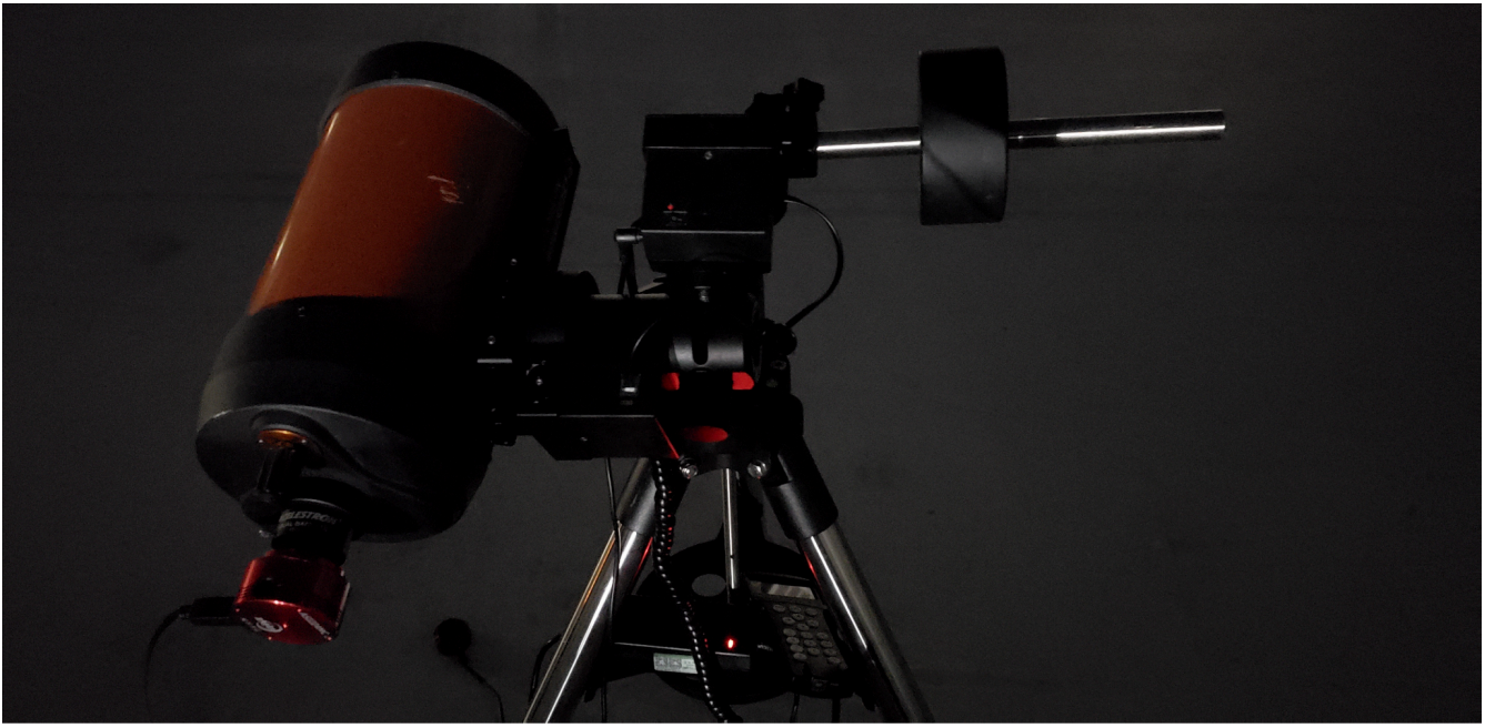
Figure 13: Equatorial Mount Balancing Position for both Right Ascension and Declination. Note that we assume the vertical Z position is already balanced, which is true for the Exoplanet Watch setup and is generally true for any telescope that is symmetric about the dovetail
