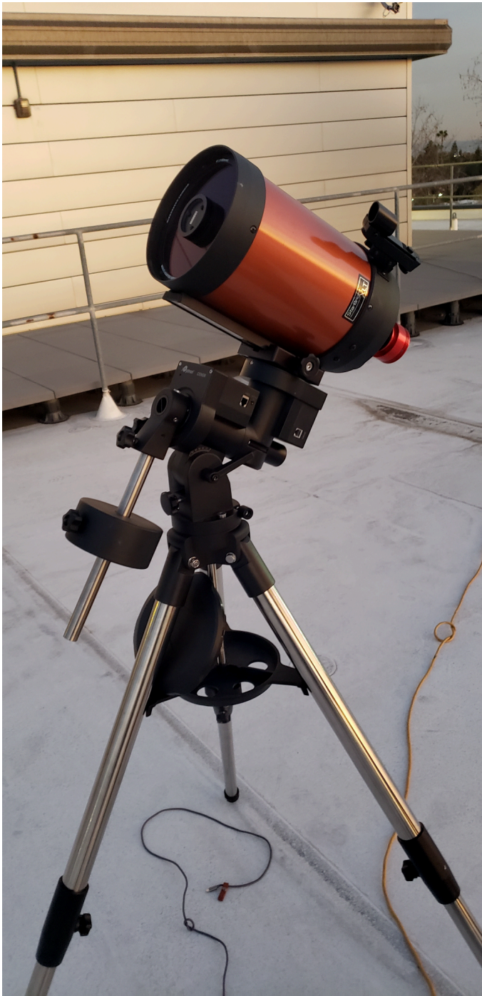
Figure 12: A fully assembled Exoplanet Watch setup ready to begin observing. Note that the tripod legs are fully extended to give room when Polar Aligning, the counterweight is properly positioned to balance the weight of the telescope tube, and the telescope itself is properly positioned on the dovetail mount.
