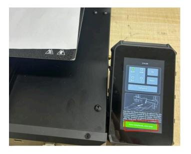
After making the first Z offset adjustment, click "First completed,next step".
