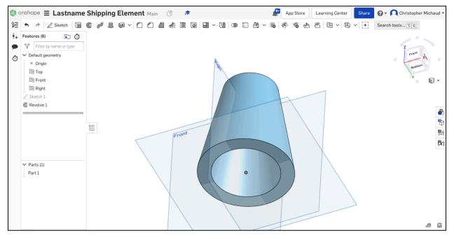
9. We are now going to add a cube to the top of the shape to put the vision target. Rotate to the top of the shape and right click on the top circle and select "New Sketch"
