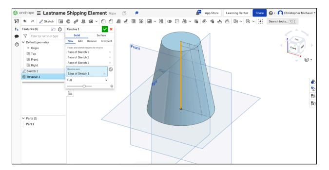
8. Click the green check mark to accept the revolve. Note that the bottom of the shape is open so these team markers can stack on each other.
