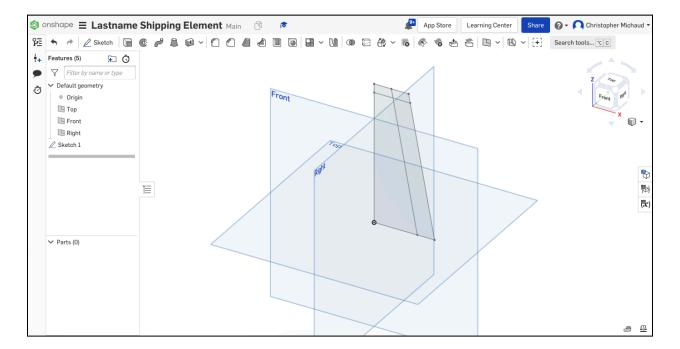
6. We are now going to use the Revolve Tool. The Revolve Tool rotates a shape around an axis. Click the Revolve Tool (to the right of "Extrude"). Then select the faces on the top and right of the shape.
