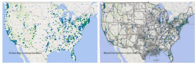
The image on the left shows the locations of those 2,200 reports. The image on the right has the same 2.200 reports and is overlaid with the 2009 EIA US natural gas transmission pipelines map. The red lines are the addition of material updates from PHMSA.
