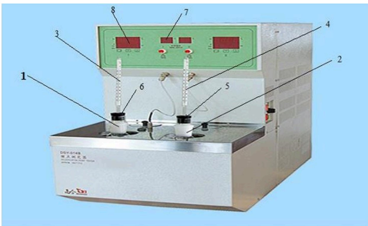
Figure 1. Determination of the cloud point and pour point of petroleum products
