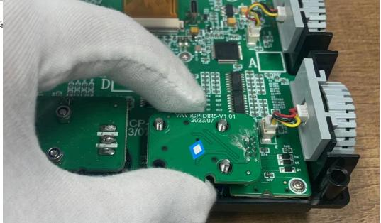
8.Ensure that the male pins align with the female connectors, taking care not to tilt or misalign them.
