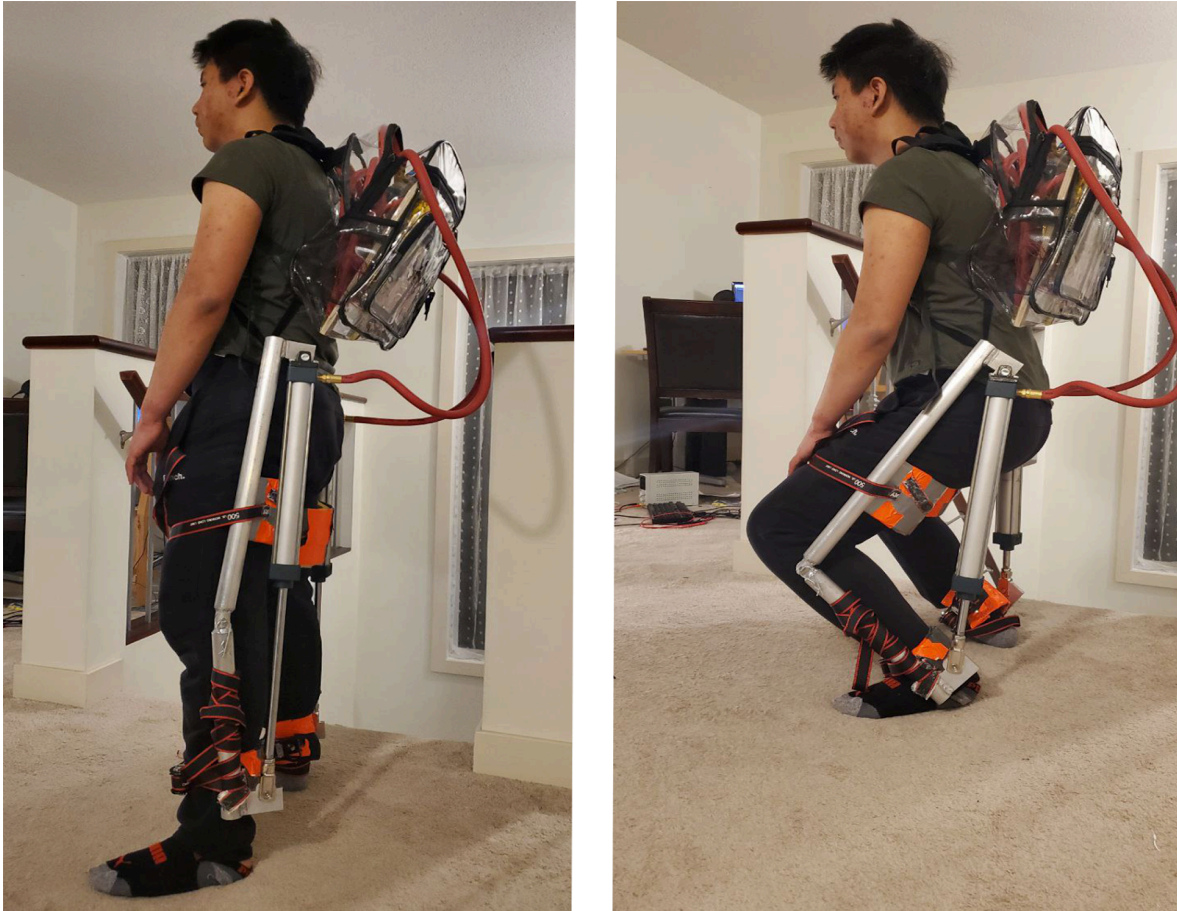
The exoskeleton shown in both fully extended form and fully squatting form.
