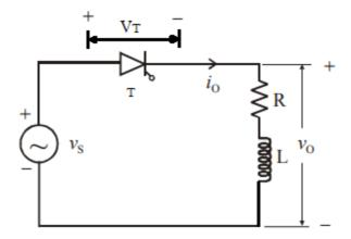
• The SCR "T" is turned ON at phase angle  $\alpha$  called as firing angle. Because of the load inductance, it continues to conduct even after  $\pi$  i.e. even after supply voltage goes negative. The back e.m.f. generated in the inductor maintains the load current in the same
