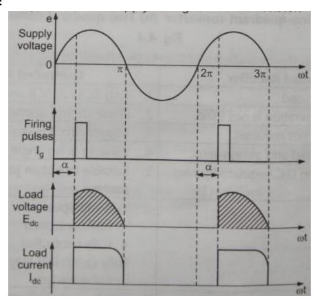
Single Phase half wave controlled rectifier with RL load
