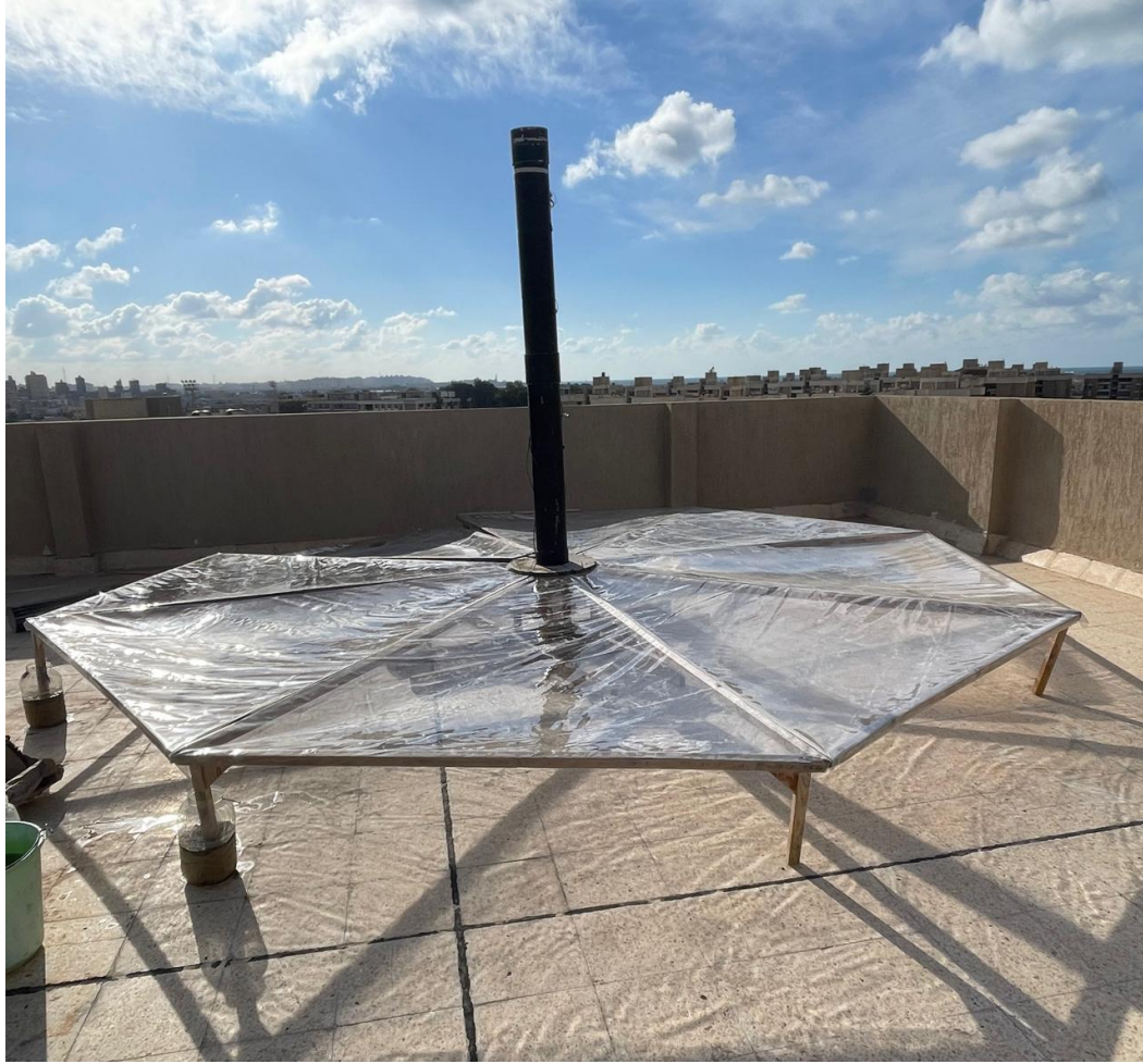
Fig 3.1 Experimental setup of Solar Chimney Plant
