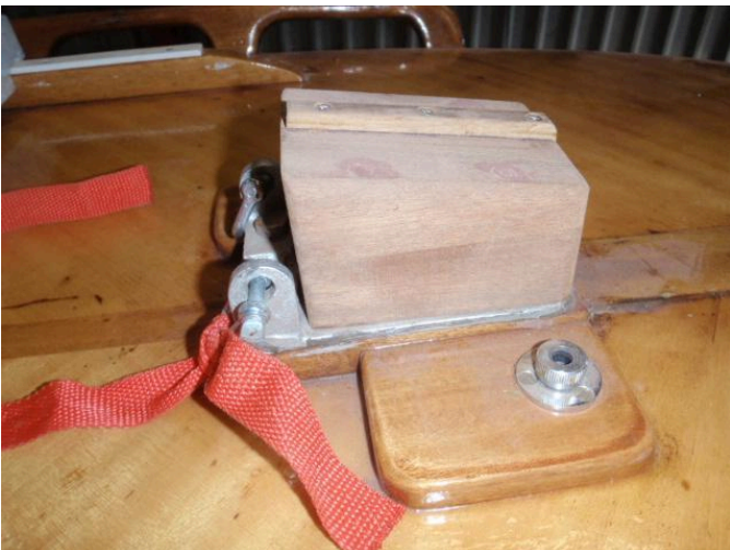
A block made to fit over the strong point of the mast step to be one of the weight bearing supports for the mast.
