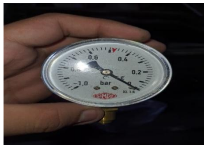
Figure 3.3.8 negative pressure gauge
