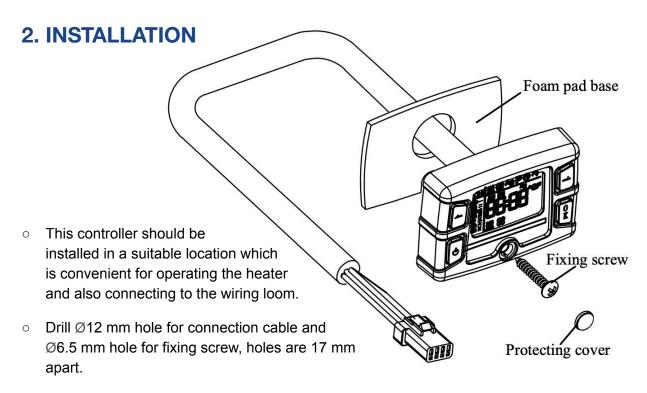
Stick the foam sticker to the mounting surface, push the cable through a Ø12 mm hole. Remove the other side of the sticker and stick the controller to it. Expansion plugs of the controller are now in the Ø6.5 mm hole. Insert the fixing screw and place the protective cover over it.
