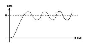
avoid overheating of the heated space. The unit then waits fully off and initiates the next heating cycle again once the room temperature drops a few degrees below preset temperature. The controller allows cycling to maintain a relatively stable room temperature.
