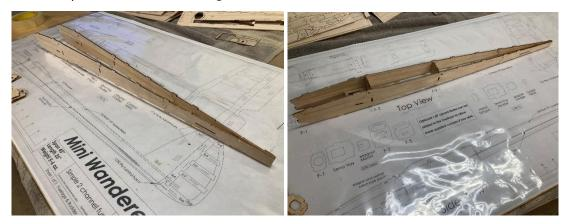
5. Working forward, dry fit F-2, servo tray and finally F-1 in place. Using a rubber band around the nose helps hold everything together before you glue. Once you have everything lined up square and straight, glue the fuselage sides together at the tail, F-3, F-2 servo tray & F-1
