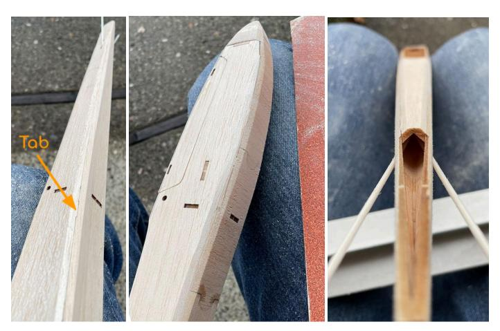
You can sand the bevel until all signs of the corner tabs have been removed. (See arrow above) In the last photo above you can see we still have a lot of material left.
