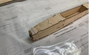
10. <u>If you intend to fit an electric motor, see the addendum elsewhere in this manual.</u> Locate and bond the stacked nose blocks in place as shown.
