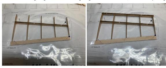
10. Laminate the two tip blocks, and bond in place.
