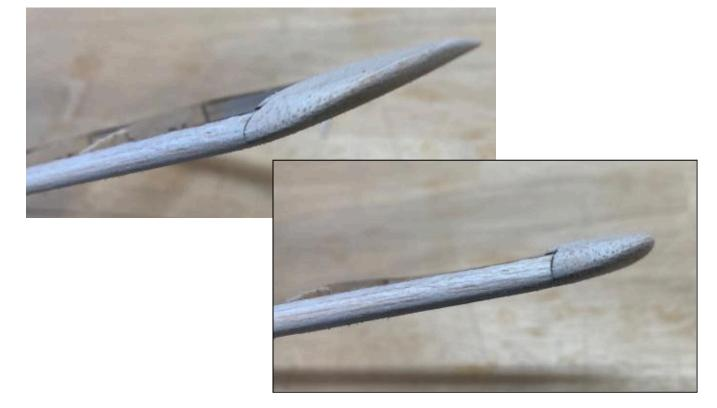
16. With the inner panel pinned flat, block the tip up to achieve 2" of polyhedral measured at the bottom of R-6. Sand the inner/outer joints so they match for a good bond. Pin the second wing right behind it so you can match the angles precisely. Bond with medium CA or epoxy.
