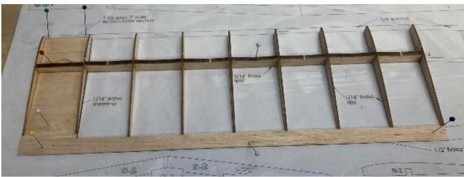
5. Using a couple pins ahead of, but not through, pull the bottom sheeting up to contact the bottom of the R-1 ribs as shown. Bond in place. Once dry sand any excess sheeting flush with the front edges of the R-1's.
