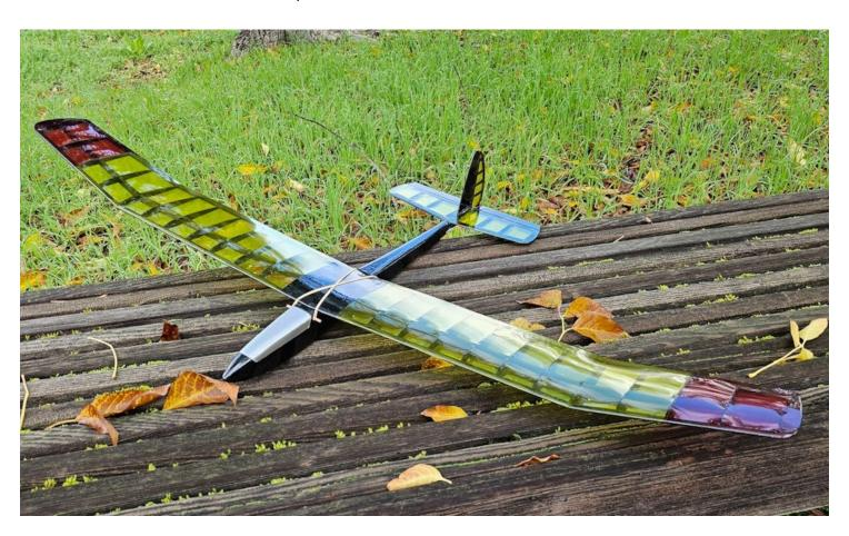
Specs: 2-3 channel (Rud/Ele/Throttle) 45" wing Span 224 Sq. In. 5-7 oz. Flying Weight
