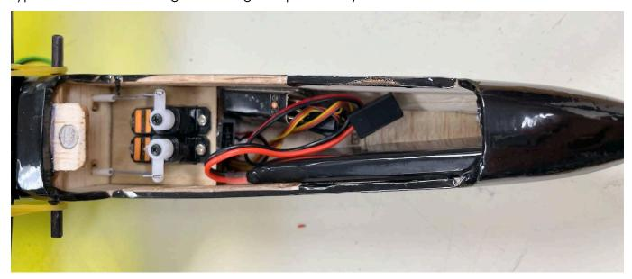
Typical radio install for electric version using micro receiver:
