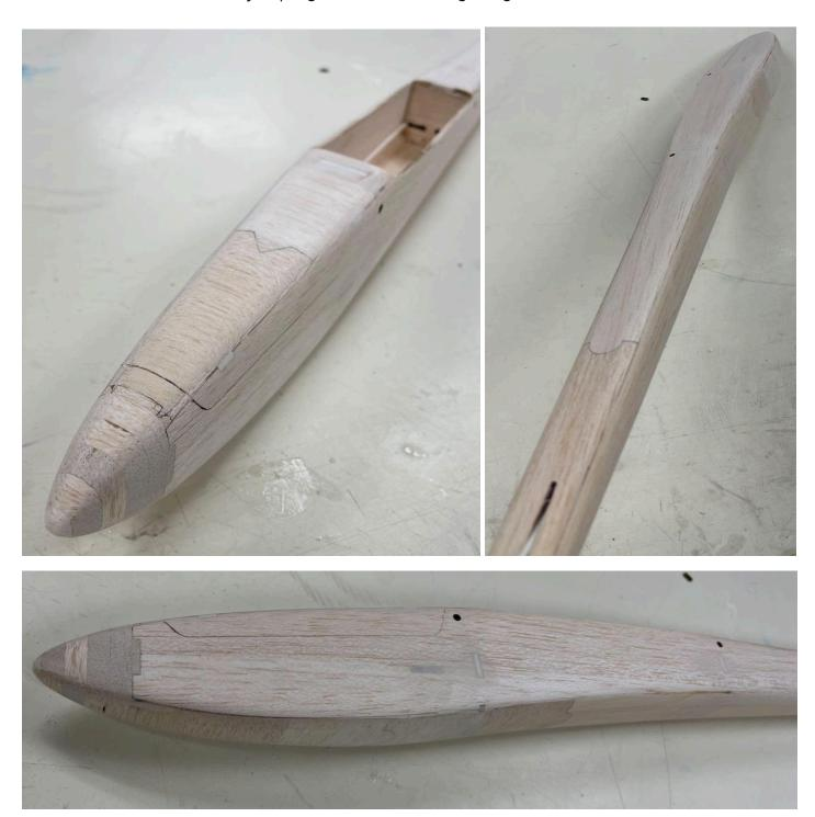
We like to fill any voids with some scrap balsa or light weight filler as seen above. It is then ready for final sanding with 320 grit prior to covering.
