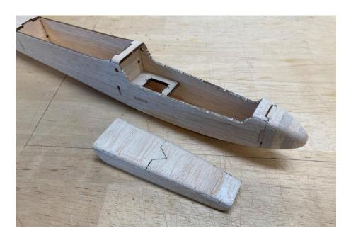
4. Locate the hatch mount, mount reinforcement (ply) hatch tongue (ply) magnet and washer. Laminate the hatch mount and reinforcement, bond the magnet in place with Medium CA.
