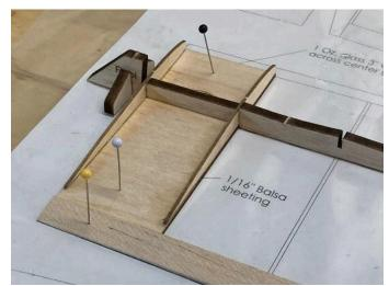
Do not glue bottom sheeting forward of the spar to the ribs, that will be bonded in the next step.
