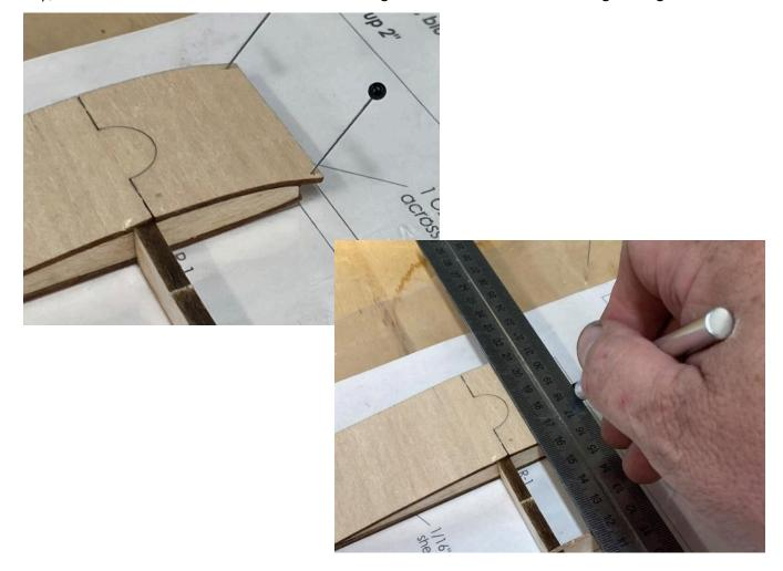
7. Fit the leading edge in place making sure it is well centered on the ribs and bond. You can now remove the right center panel from the building board to make room for the right tip.
