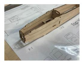
6. Locate the bottom sheeting pieces. Starting from the rear, fit the sheeting in place and bond. Care must be taken to not introduce a warp at this point. Continue with all of the bottom sheeting.
