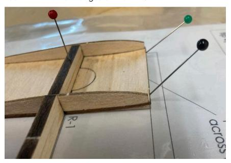
6. Assemble the 2 pieces of the top sheeting and bond in place as shown using pins. Once dry, trim the excess flush with the F-1's using an x-acto knife and straight edge.
