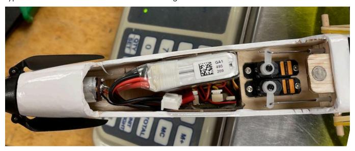
11. It is very important to adjust the Center of Gravity (CG). The **CG** is located on the spar at the sides of the fuselage. For beginners we suggest first flights with the CG near the front of the wing spar. You can slowly move the CG back each flight until you have found the point you like the most. At the rear of the spar the Wanderer should perform nice loops without much effort.
