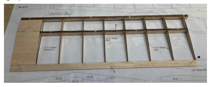
8. Pin the right tip spar in place over the plan. Using the TIP dihedral gauge, set R-2 in place at the proper angle. Add R-3 through R-6 but do not glue.
