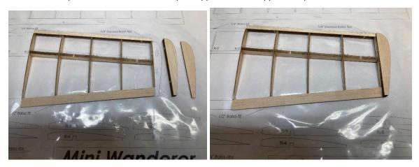
11. Remove the right tip panel from the board and repeat the above steps for the left center and tip panels.
