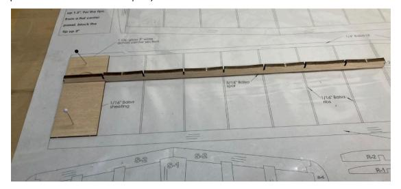
3. Locate the Root and Tip dihedral gauges & assemble. Using the TIP gauge, set the last R-2 in place, but do not glue yet. Fit the ½" trailing edge stock and pin in place behind F-2 and bottom sheeting.
