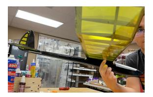
12. The electric version will be very close to CG depending on your radio gear. CG should be able to be adjusted by battery location when using a micro receiver. The electric motor is designed for a 2S 450mah lipo battery. The recommended Emax servos are limited to 6 volts, so you may need to add a BEC to limit voltage to the servos as many micro receivers do not offer this. Aloft offers a micro BEC that works very well for this.
