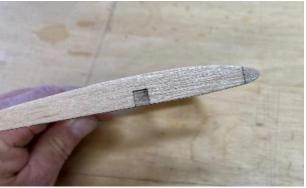
14. Rough shape the wing tip with 80 grit on a block. I like to sand from the bottom up following the natural contour of the airfoil. Leave about 1/16" of the laser etch line as a guide.z
