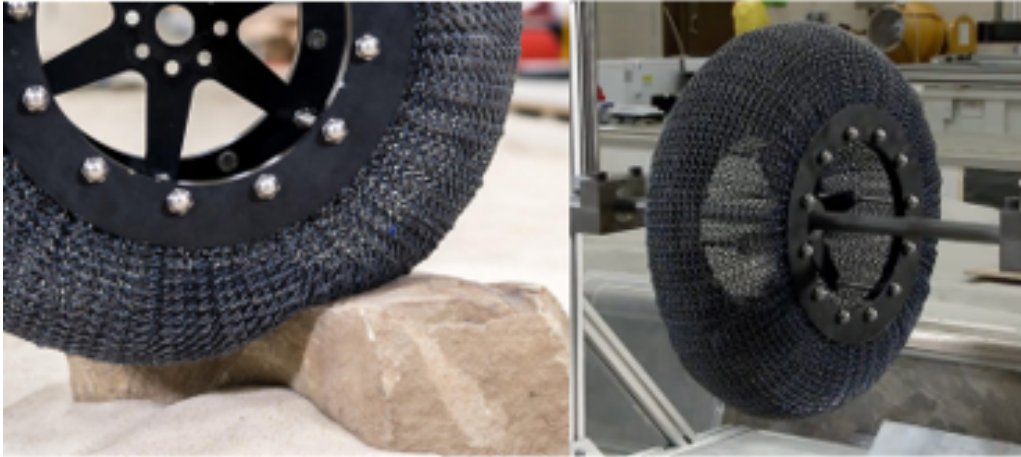
Figure 7: Mesh Wheel Inspiration from the Lunar Rover [2]
