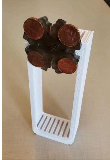
Figure 20: Test Bed with Flywheel Attached by a Motor
