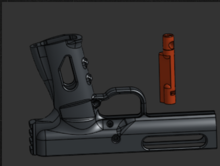
5 walls, 20% infill, Supports everywhere, 85° overhang angle
