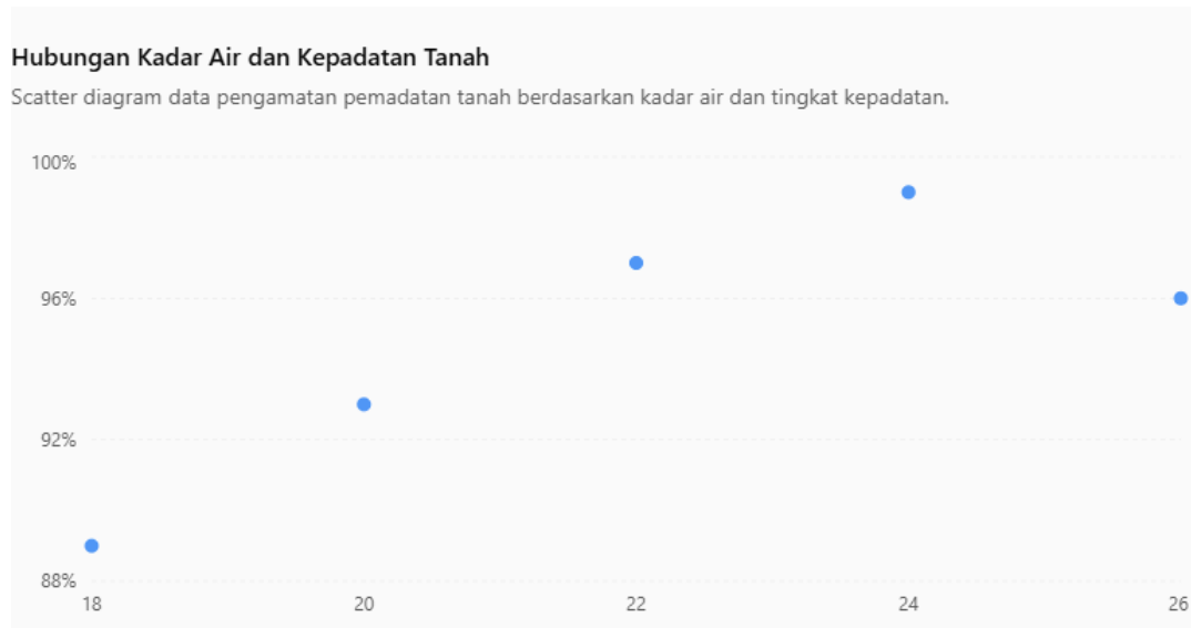
Gambar 9.11 Scatter Diagram Kadar Air vs Kepadatan Tanah
