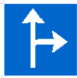
E11.7 Hanging arrow traffic sign. The sign indicates the driving directions for the lane under the sign.
