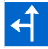
E11.6. Hanging arrow traffic sign. The sign indicates the driving directions for the lane under the sign.
