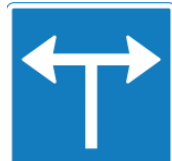
E11.8. Hanging arrow traffic sign. The sign indicates the driving directions for the lane under the sign.
