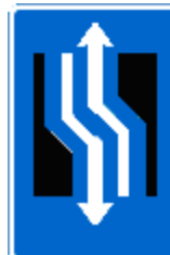
E16.3.13. Continued to the left and with oncoming traffic
