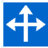
E11.9. Hanging arrow traffic sign. The sign indicates the driving directions for the lane under the sign.
