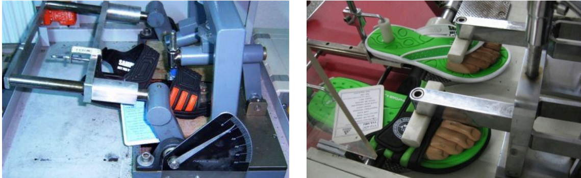
Figure 1: Sandals/Slides flexing machine
