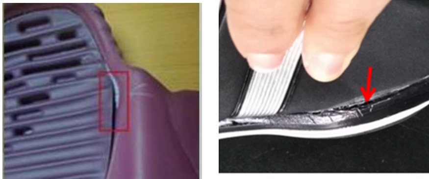
Figure 4: Failure examples of delamination and outsole cracking
