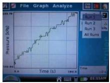
We know from our math classes that the line in this graph has an equation of y = mx + b. For our purposes, we only care about m, the slope of the line. The slope, or steepness of the line, tells us how quickly the gas pressure is increasing. The steeper the line, the greater m will be and the more oxygen is
