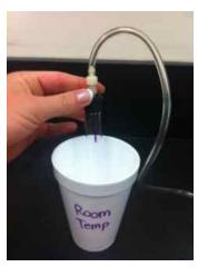
12. Start data collection by pressing the green play icon. Data collection will stop after 3 minutes. (Monitor the reading on the screen. If the pressure exceeds 130 kPa, disconnect everything and start over with less enzyme solution.)
