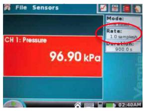
9. Change the data-collection rate to 0.5 samples/sec and the duration to 180 seconds. Press OK.
