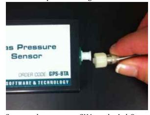
7. Connect the sensor to CH1 on the LabQuest.
