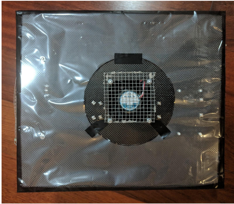
The bottom of the device, with the skirt and fan visible.
