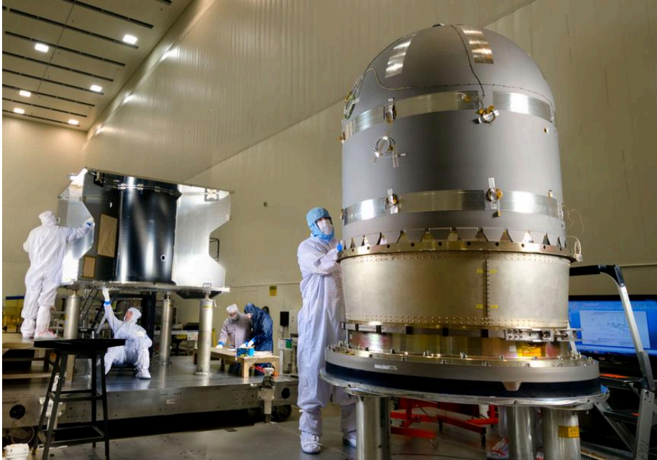
The large hydrazine propellant tank prior to integration with the core structure of the MAVEN spacecraft at a Lockheed Martin clean room near Denver. Image Courtesy of NASA.
