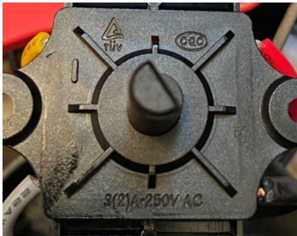
Top of switch with knob removed
