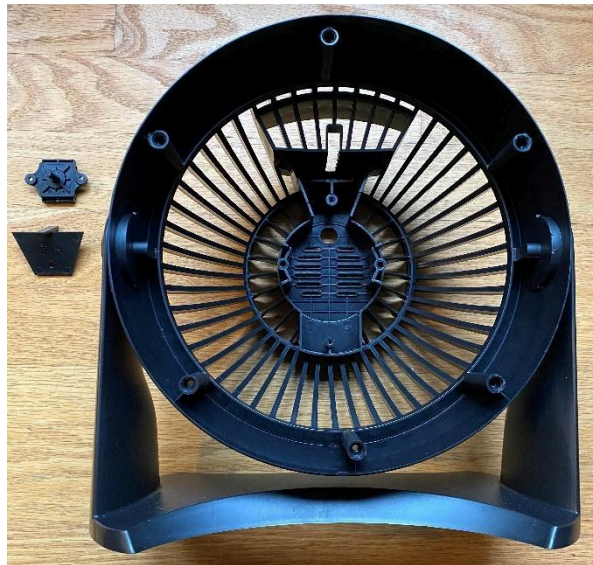
Empty fan housing with power cord removed
