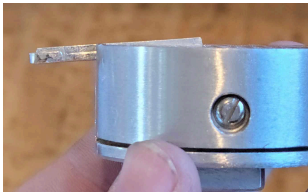
Fig. 13 - Clasp pin held in my hand vise for shaping into a point.
