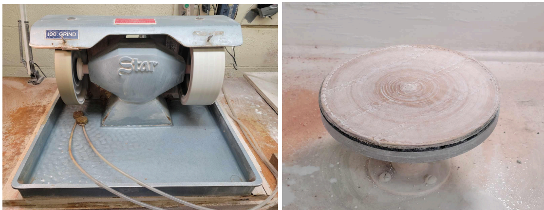
Fig. 3 - Left, the cabochon machine used in this project. Right, the flat lap with a leather top used for oxide polishing.
