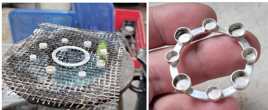
Fig. 8 - Left: each component has the cleaning solvent burned away before soldering. Right: after soldering, thankfully all in one well-bonded piece.
