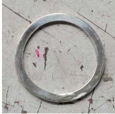
Fig. 6 - The finished ring, to which the bezels will be soldered.
