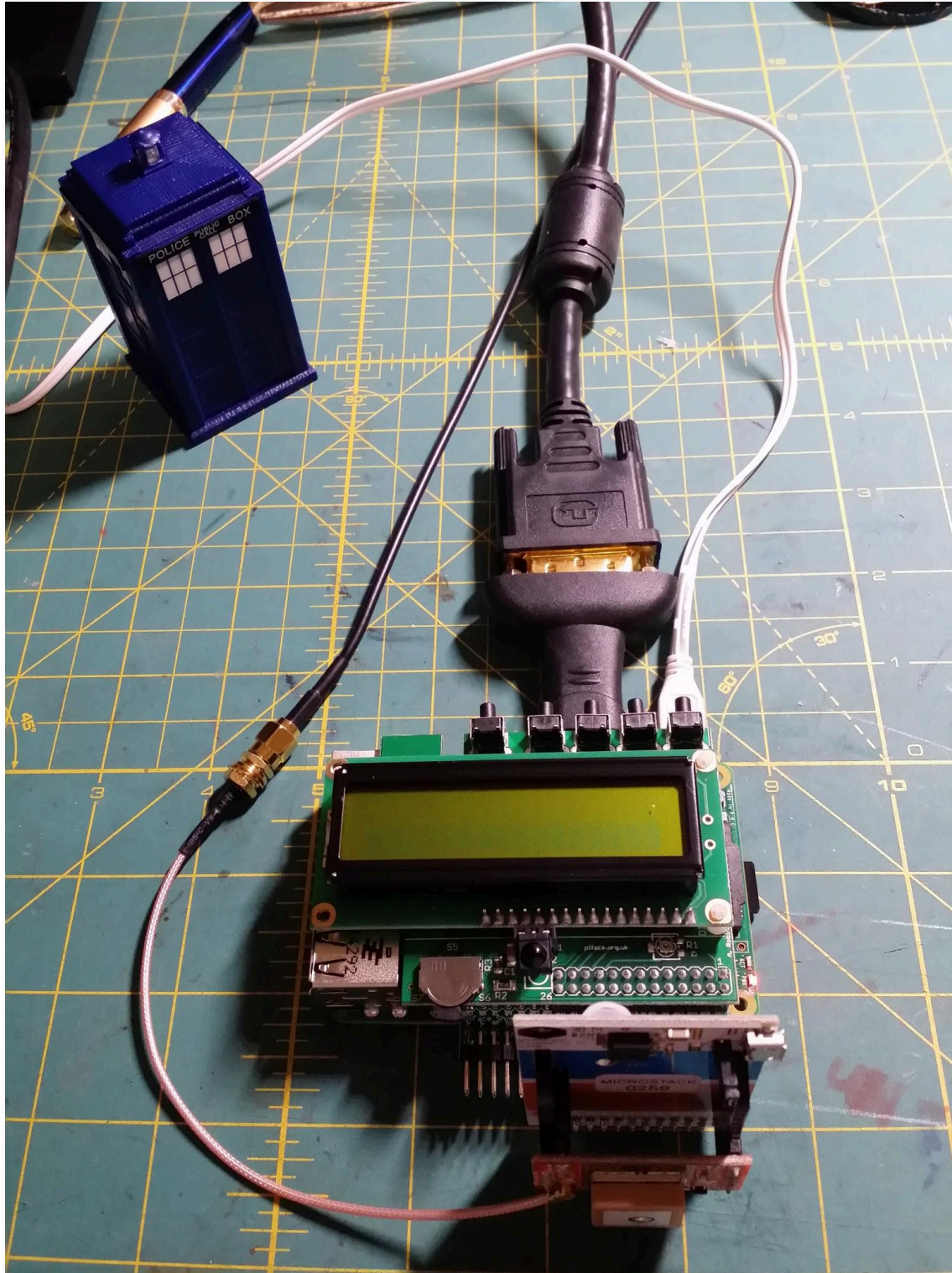
Ready to power up! Note the DVI-HDMI adaptor for my DVI only monitor.
