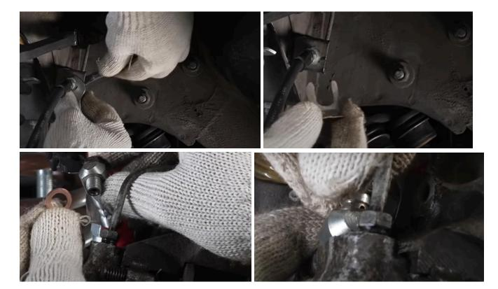
Connect the hose to the caliper with a standard banjo bolt with copper rings.
