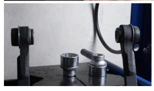
Install the lower ball joints of the VAZ 21214 into the upper arms. The bolt heads must be on the ball joint side.
