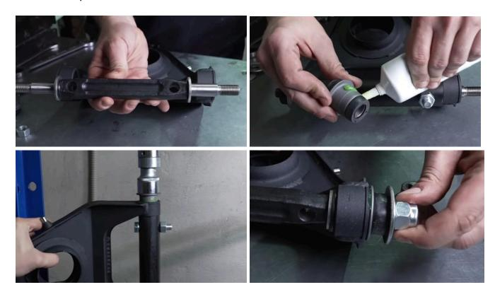
**Attention!** Ball joints are installed from below the control arm. Bolt heads should be on the control arm side, so you do not damage the ball joint boot.
