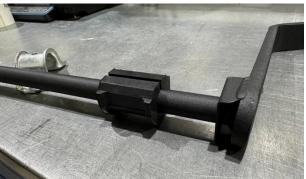
Screw the stabilizer to the adjustable brackets on the car body with the VAZ 2108 stabilizer brackets. Use the bolts and nuts from the kit.
