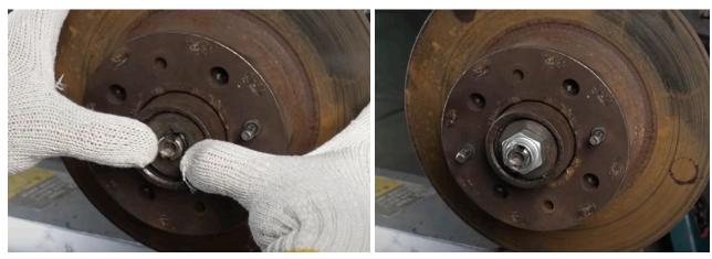
Install the hub with the brake disc and secure with a nut.
