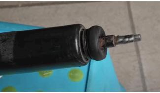
Make sure that the shock absorber rod fits into the hole in the body.
