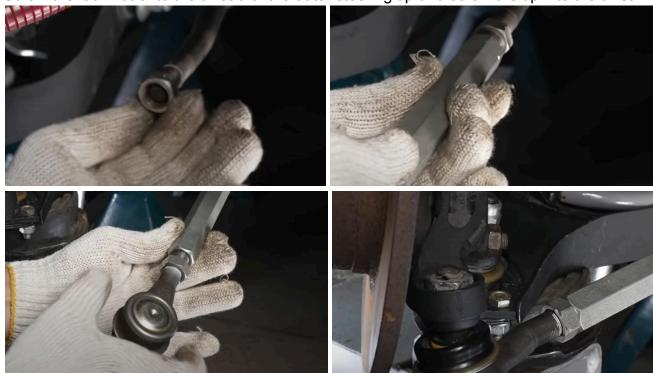
Insert the steering tip pin into the steering arm bushing. Screw in and tighten the tip nut. Do not tighten the steering rod twists and their locknuts yet. This should be done after the car is on its wheels and at least the approximate toe-in of the front wheels is set.
