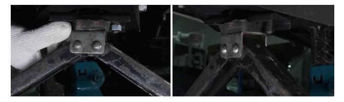
Using the jack as a support, press the shock absorber bracket against the control arm until it is completely seated on the studs. Secure the bracket with Grover nuts.
