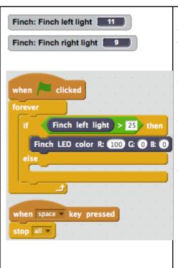
**#1** If **Finch left light** detects the flash light, its beak turns red. This conditional logic is implemented with an **if-else** block. The **if** condition is a **comparison expression**
