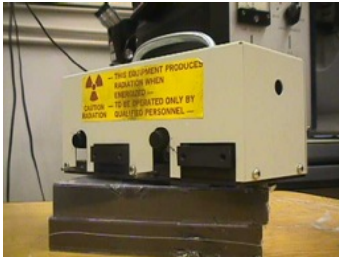
10.5 Bartels four-bounce monochromator.
