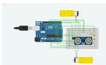
During the creation phase, my teammate and I started to design the physical structure of the robot using ThinkerCad by utilising the available tools and components in the ThinkerCad library to create a virtual representation of the robot's body. Furthermore, we were also able to code the entire robot within ThinkerCad in C++, which allowed us to test if our design/plan would actually work before building the prototype of
