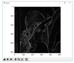
(2) Image – Erosion (internal gradient)
