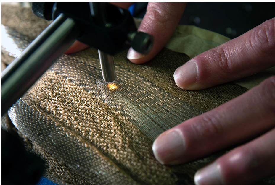
Scanning_fibers.jpg : Brian Iezzi scans and measures the photonic fibers in the fabric he developed. Photo: Marcin Szczepanski, Michigan Engineering
