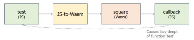
If we just inline the JS-to-Wasm wrapper, we can handle this case with a specific lazy-deoptimization builtin, which is called by the Deoptimizer to complete the work of the wrapper before resuming execution of the caller function in the interpreter.
