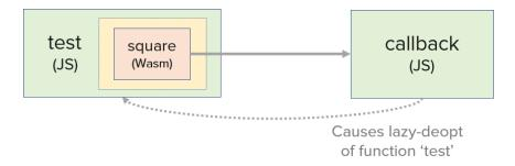
In this case we will have a call to a Wasm-imported callback function from the inlined Wasm code. At the end of this call the compiled caller function should be deoptimized. But from where should execution resume, in the interpreter? If we resume from the JavaScript code that immediately follows the Wasm call, we skip all the code in the Wasm function after the callback.
