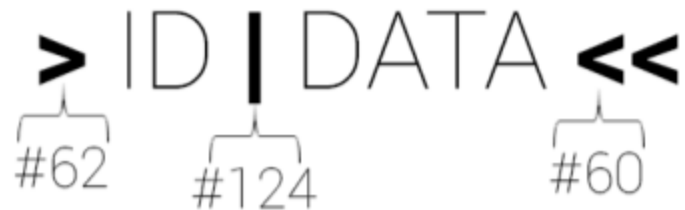
Fig 1. A Hermes packet. Note the characters used to define the packet structure are in bold and show their associated ASCII values. The user sets the ID and DATA fields.
