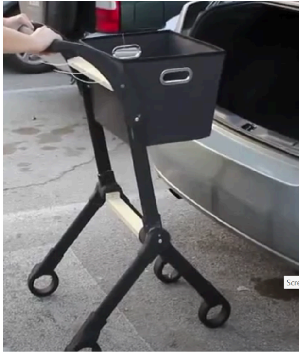
Figure 18: The upright position of the foldable shopping cart.
