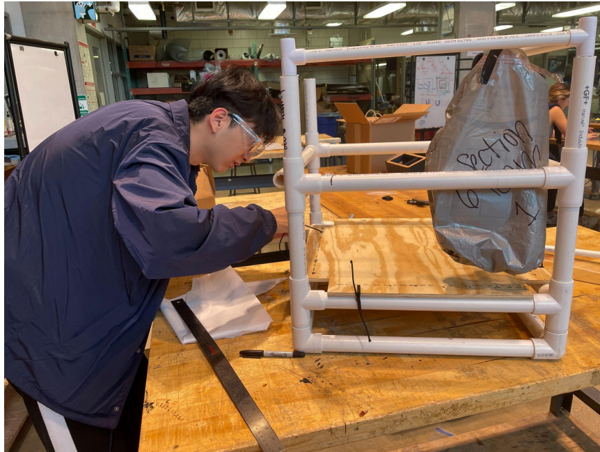
Figure 47: Connecting the plywoods with the PVC pipes using nylon ropes
