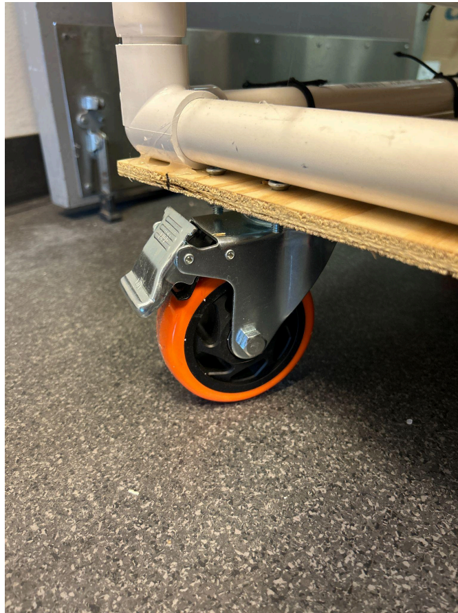
Figure 11: Wheel in Locked Position
