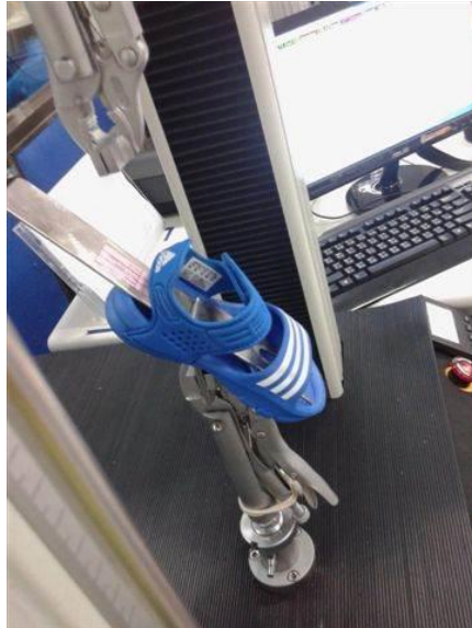
b) Tool + shoe fixed into the lower clamp
