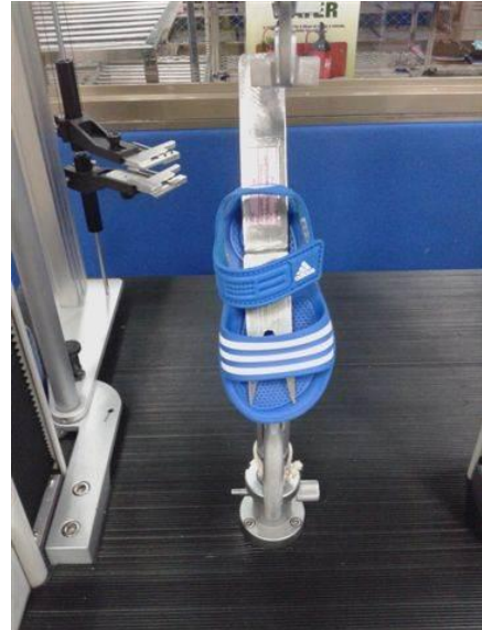
b) Tool + shoe fixed into the lower clamp
