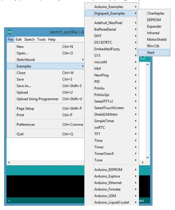
Since <u>CuteDuino</u> use Digispark bootloader, we need to select **Digispark** (**Tiny Core**) as Arduino **Board**.
