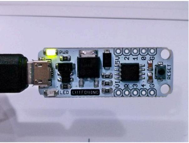
For the first time connection, computer will not recognize <u>CuteDuino</u> (Unknown device).
