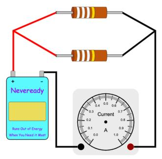
Step 2: Find the resistance of your resistors based on the color code and then find the total resistance of the combination of resistors. Show how you did this in the space below
