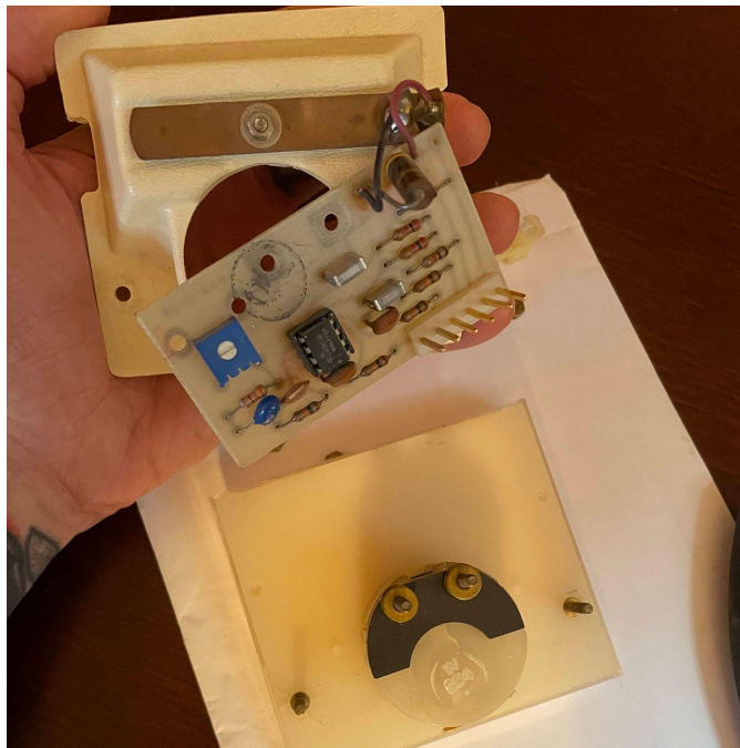
Housing and meter buffer removed from meter.
