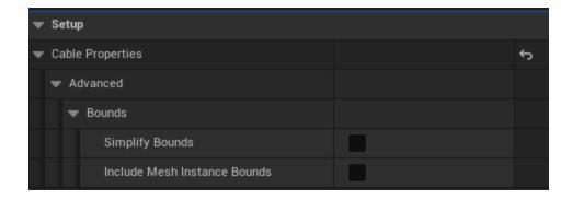
**Simplify Bounds**: Uses faster bounds calculation by only considering start, middle and end points of the cable therefore calculated bounds may not be accurate. This may affect shadow casting as well. only viable when the number of particles is high.
