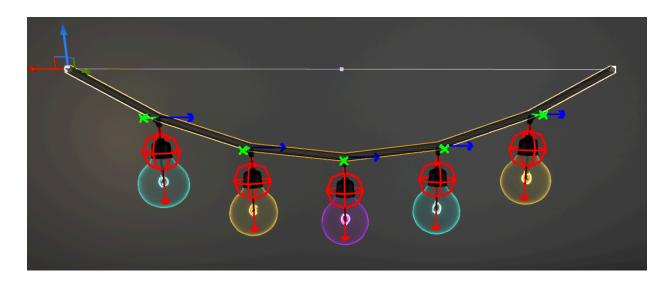
Enabled: Hanging lights are still simulated but these light bulbs can only rotate around their Z axis.
