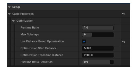
**Runtime Ratio**: Lower values can reduce the simulation cost. value of 0 will halt the simulation (does not disable the component tick). default is 1.
