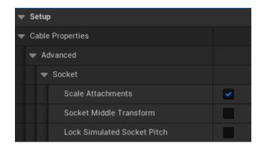
**Scale Attachments:** if true, sockets and attached mesh instances will be scaled by the string light component. call <u>Mark Render State Dirty</u> after changing this option from the blueprint.
