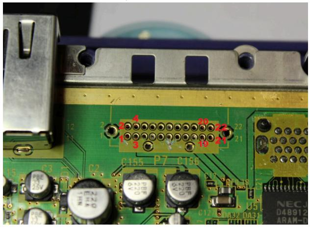
13 signals need to be connected from the digital video port to the Pluto board. Please make sure that the wires are kept short as you are dealing with high-speed digital signals here. The pins on the Pluto board are labelled on both the top and bottom sides.
