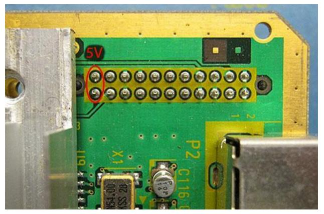
Either of the marked pins (they are already connected together on the Cube's board) must be connected to the VUNREG solder pad on the Pluto board. If the image is unclear, the two 5V pins of the power connector are the two pins closest to the heat sink.
