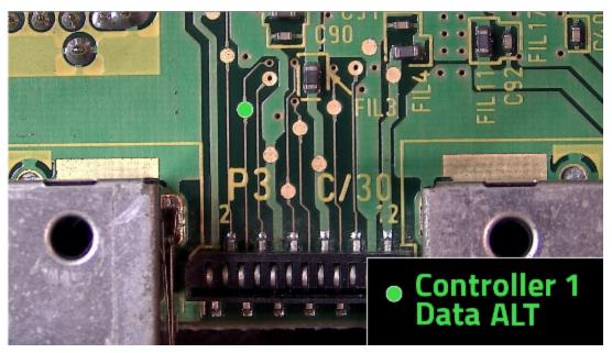
To read the controller buttons, another wire must be connected from the FPGA board to the Gamecube. The recommended connection point for this is on the bottom of the Cube's PCB, it must be connected to pin 94 on the Pluto FPGA board.
