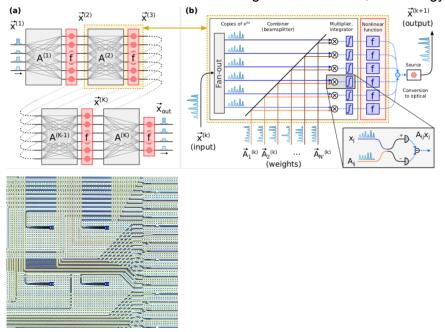
Left: a deep neural network decomposed into layers (activations plus matrix-vector multiply). Center: schematic of ONN based on coherent detection [3]. Right: false-color image of part of an ONN circuit.
