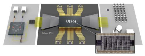
Illustration of the silicon "quantum photonic processor," which includes entangled photon pair sources (left), unitary state evolution (center), and a bank of superconducting detectors (right).
