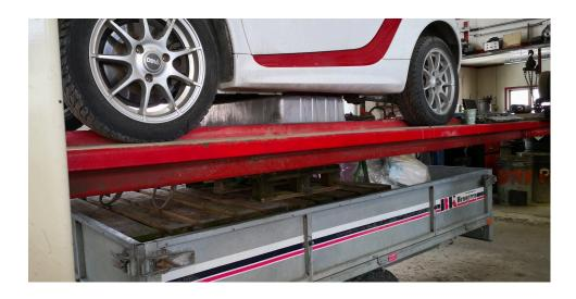
Removed all nuts under edge and drilled out rivets. Removed torx around connectors. PS! The vent hose connector must be removed by a unbrako key (at the right on this picture).
