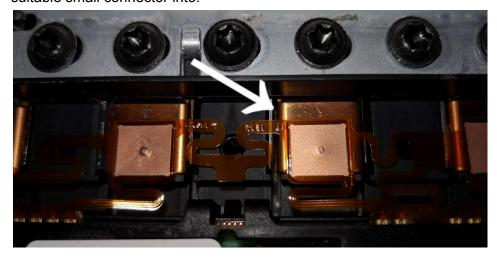
But on the outer cells, there is no gap, so I ended up with a clip with pressure from a piece of wood (Remember NO METAL OBJECTS....). (If I had more time I would have made something more elegant than this quick fix..)
