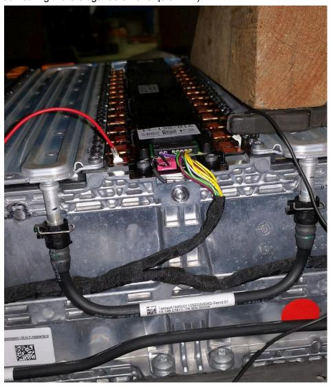
Be aware of extremely fragile point weldings of the cell monitoring connectors. One of mine came loose, so I had to repair the connection by soldering it.
