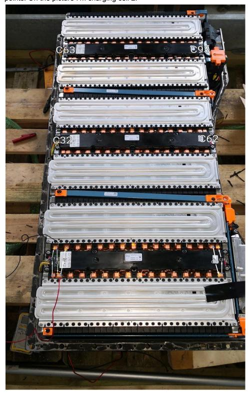
To charge one cell at a time, I simply used a 45W USB-C PD that also have a 5V USB connector capable of 2.4 Amps:
