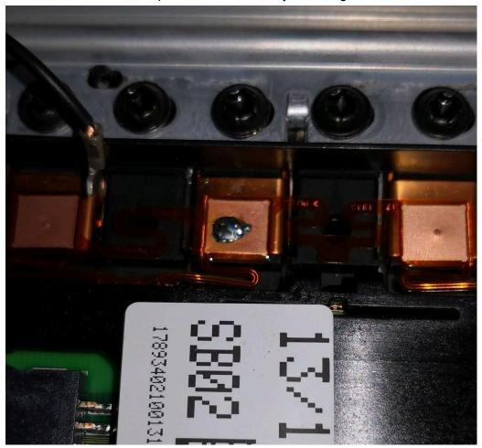
After all low cells were charged up to approx 3.35v and stayed above 3.3V for some hours, everything was put together and fitted to the car. And the two errorcodes went away by themselves so standard charging from 220V AC mains could be started directly afterwards.
