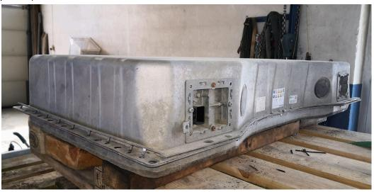
Cover is glued tight. I used a tiny chisel and a hammer all the way around. BUT PAY ATTENTION. BATTERY CELLS ARE CLOSE BEHIND, SO DO NOT GO DEEP !!!!
